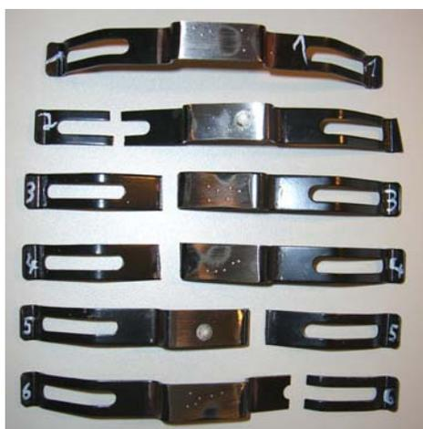
Fig. 2: The fractured third party hold-down springs
