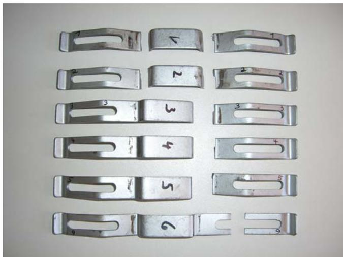
Fig. 2: The fractured third party hold-down springs
