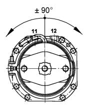
With this kit you have the possibility to turn the exhaust in the cylinder cover to the air connections with max. +/- 90°.
