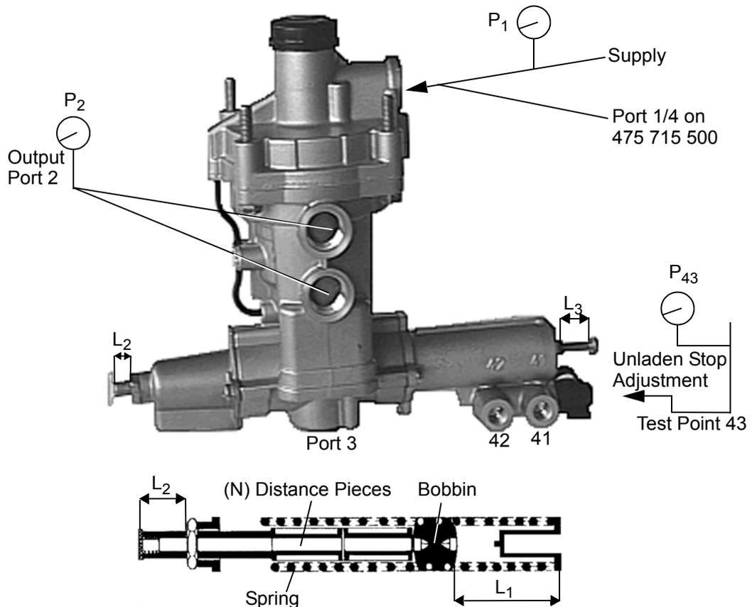
Always release ALL PRESSURE after each test, As this valve physically "LOCKS-UP" under pressure setting adjustments when pressure is applied and can cause internal valve damage.
