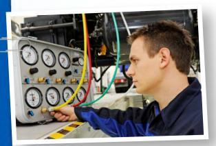
When we are repairing a vehicle with a defective braking system, it is often difficult to identify the braking part which is causing the trouble. This often takes a lot of time and increases the downtime of the vehicle. With the Mobile Test Bench this is over: now we can check in detail directly and avoid unnecessary extra repair time.
