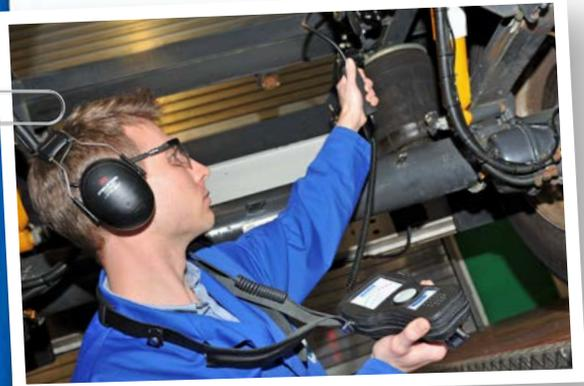
“ When a truck comes in for service, we do a two-minute routine check for leaks. On one occasion, we identified 2 smaller leaks caused by two worn out screwing connectors. To avoid further damage and costs, we repaired them. The result: a customer that was very happy we were so thorough, and some additional business for the workshop. ”
