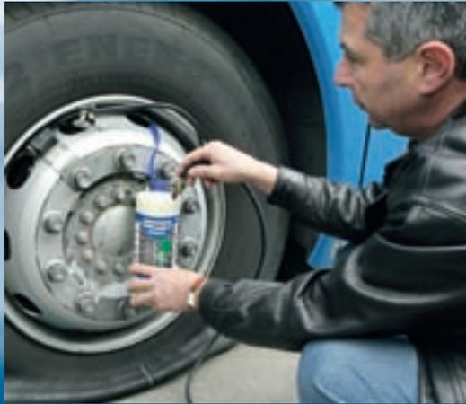
Using the truck's compressor, pump in the sealant through the valve extractor which also prevents venting.
