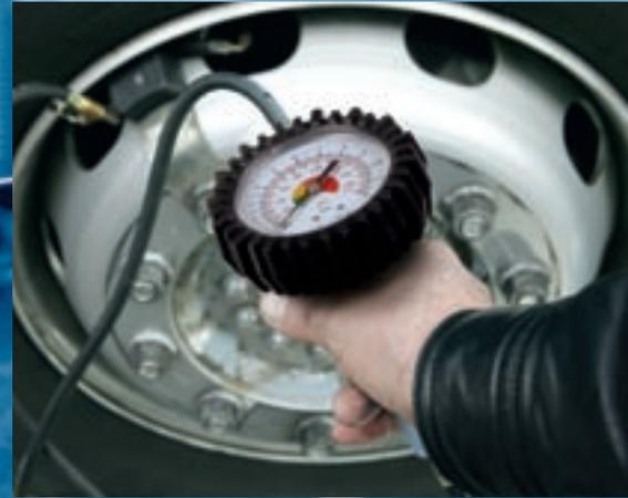
Use the kit's manometer and 10 meter long hose to periodically monitor tire pressure.
