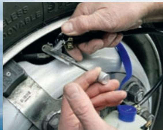
The valve extractor set lets you easily remove valves from single or dual tires without having to remove the wheel.
