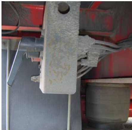
fig. Rotary slide valve with RtR function of a third-party supplier with blade terminal (left) and with DIN bayonet (right)
