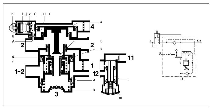
Compressed air passes from the tractor through the supply line hose coupling to port 1, passes grooved ring (c) and continues through port 1-2 to the trailer reservoir.
