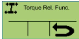
The relaxation function is activated by switching on the function in the TEBS E1 modulator. The tension on the applied brakes is released with the respective actuation of the brake cylinder from the modulator. The brakes are released by side (semitrailer/central axle trailer) or by axle (drawbar trailer) for this purpose. Braking the vehicle is always performed at over 18 %, because the brake cylinder is used for releasing the vehicle.
