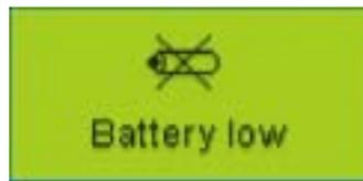
**!** If the battery voltage is no longer sufficient to operate the internal real-time clock, the menu <Extras> <Settings> <Clock> is greyed out. It is then no longer possible to transmit the time via CAN, i. e. the ODR data of the Trailer EBS E can no longer be saved together with the time.
