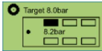
**!** The tyre symbol flashes if the tyre pressure is too low. If the tyre has a fault, the warning LED and the menu item for this functional group flashes in the main menu. Messages are only output via warning LEDs and flashing menu items if the "Event LED" functions is activated (see page 33).
