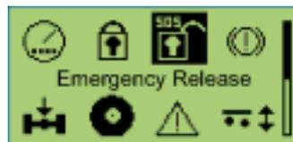
The "Emergency trigger function" menu appears if the function is defined and activated in the TEBS E modulator.
