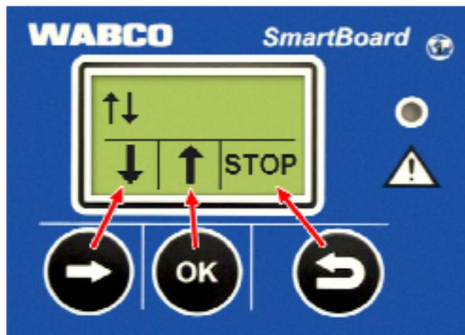
fig. 4-1: Button assignment for operating the air suspension
