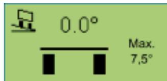
In every Trailer TEBS E1 modulator a lateral acceleration sensor is integrated for the RSS function. This sensor simultaneously provides information on the inclination of the vehicle to the body reference plane. The inclination of the vehicle can be monitored in the Trailer EBS E1 Modulator.
