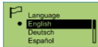
The SmartBoard is equipped with a language package. The language package can be changes in the Diagnostic Software (see chapter 6.4 "Diagnostic Software „SmartBoard“", page 45).
