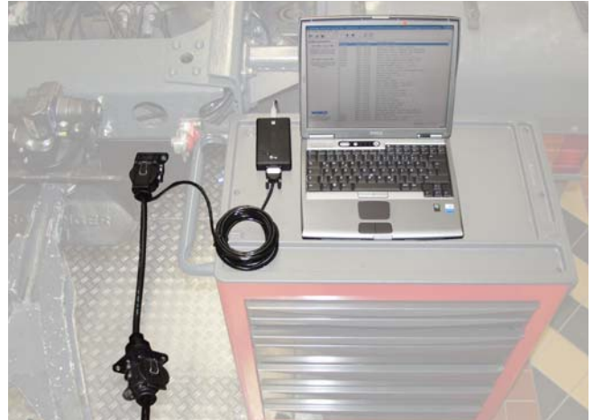
Fig. 4 Cable connection via ISO 12098
