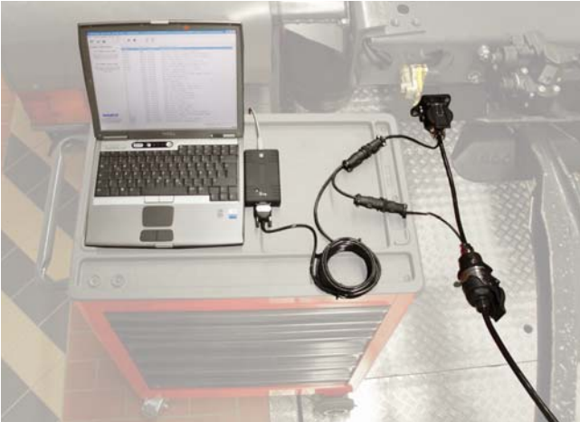
Fig. 3 Cable connection via ISO 7638
