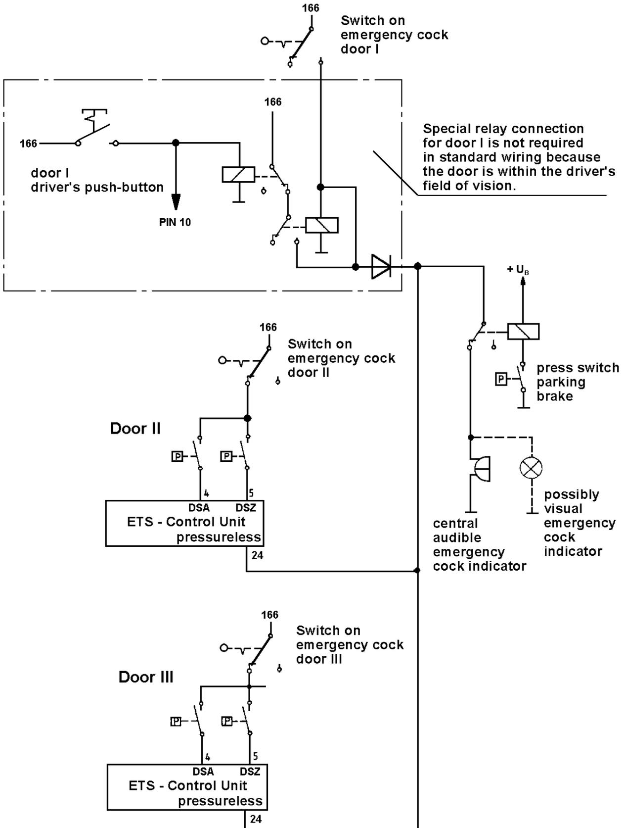
ETS ECUs 446 020 012 0 / 013 0 for Linear Drive, only Door II or III with Extended Emergency Cock Logic
