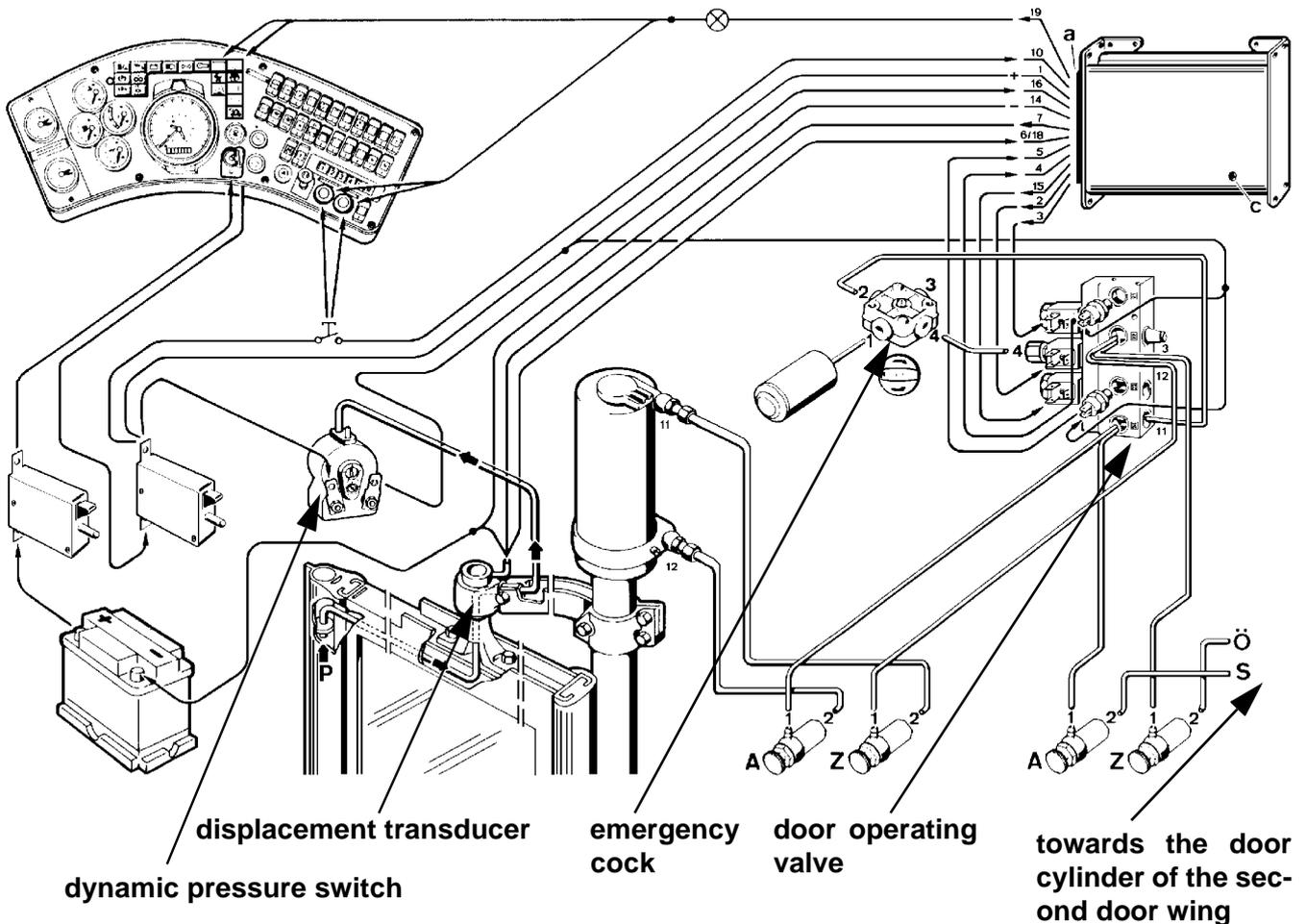
The diagram above shows an ETS door operating system and the arrangement of the door components. The system in this example has a rotary drive. i.e. the door operating cylinder is mounted directly on the heel post of the door wing.
