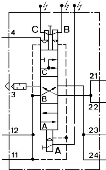
It is important to remember that - due to the different surfaces of the door cylinder pistons - the door leaves move deliberately slowly towards the open position. The driver can close the door again at any time by pressing the push-button on the dashboard.
