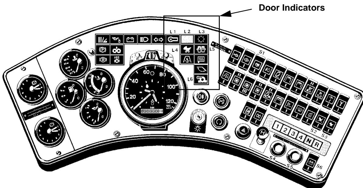
The illustration on Page 12 shows an example of the typical dashboard of an urban routine bus. Different indicators are used to inform the driver of the "condition" of the doors via the ETS ECU.
