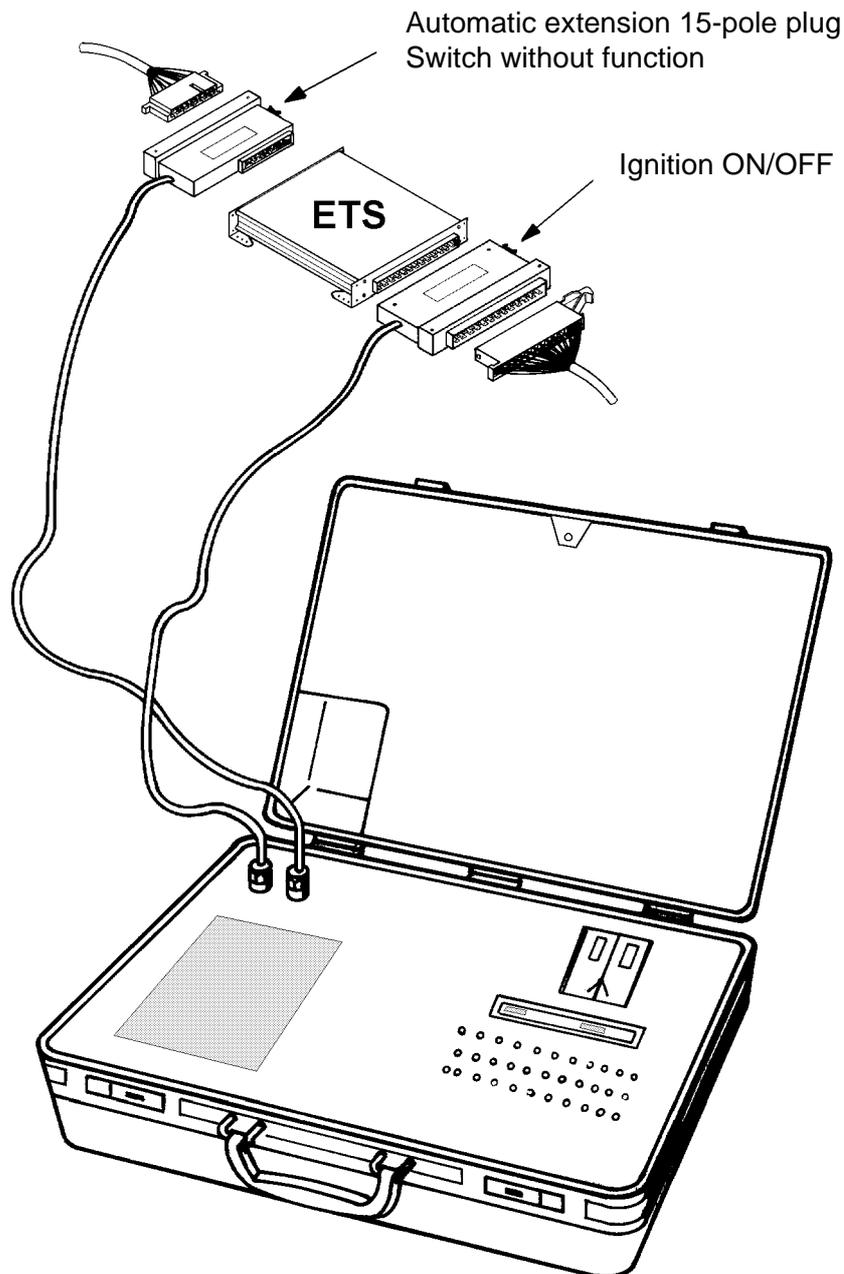
**The ETS test equipment case has the WABCO Part No.: 884 901 555 0.**
