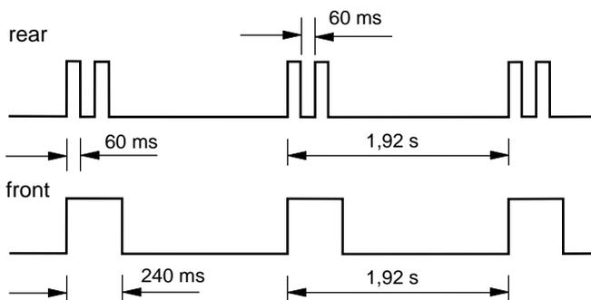
Another telltale is found inside the housing of the ETS ECU. This is a light-emitting diode (LED). When trying to locate an error, this malfunction indicator and/or the telltale in the driver's push-button are used to flash out error codes.
