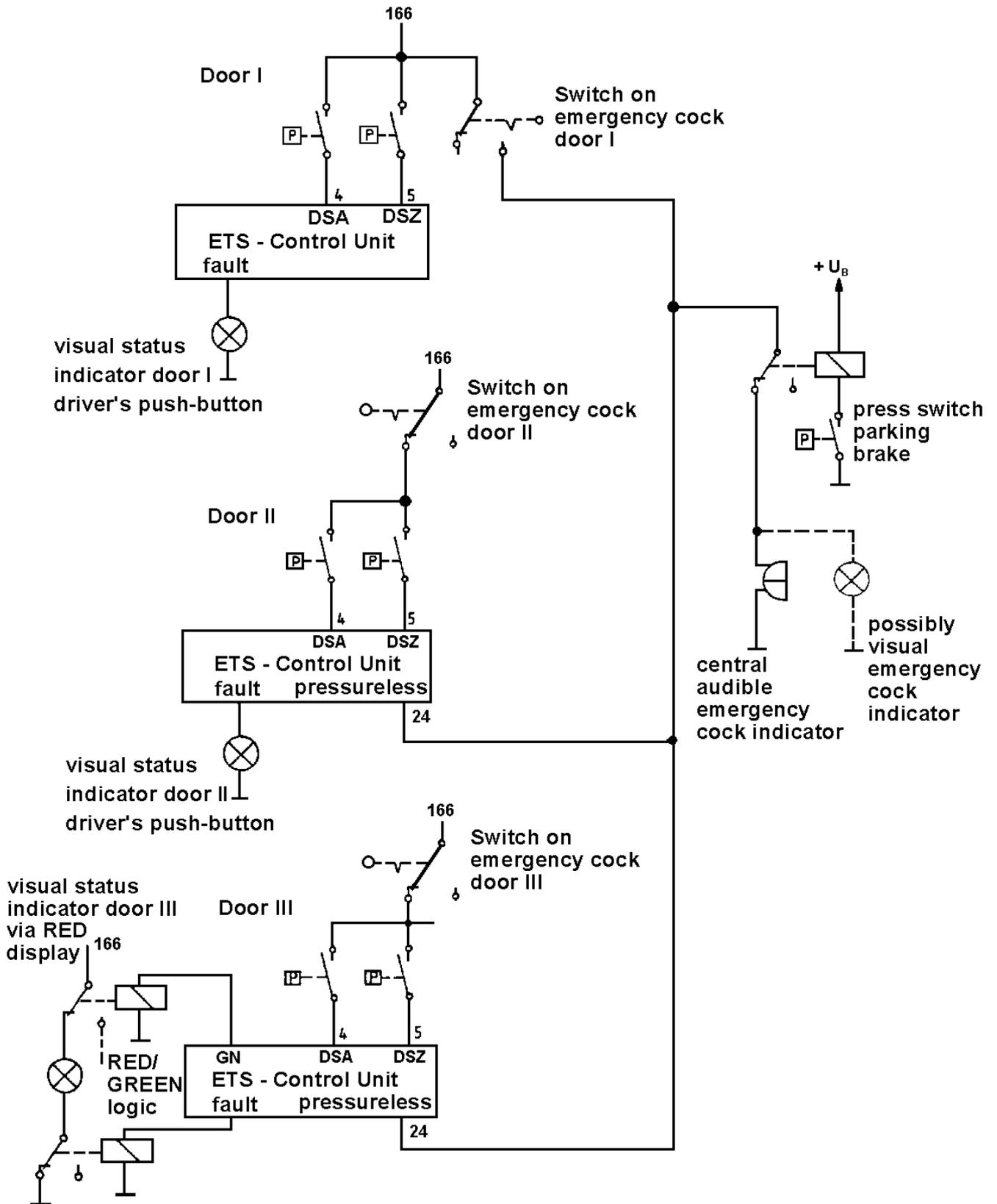
Typical Wiring for Extended Audible Emergency Cock with Additional Connections for Door I
