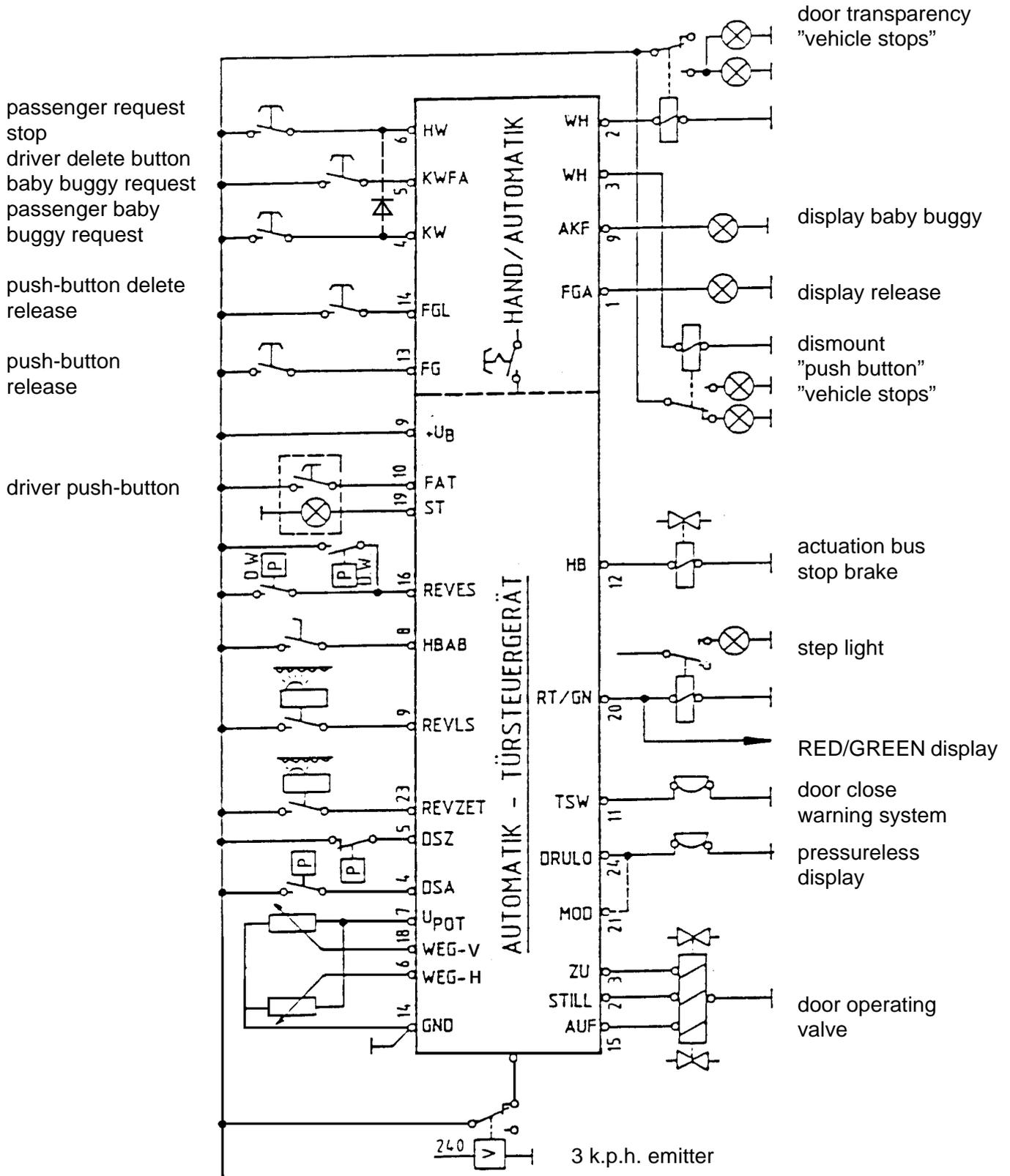
The basic ETS unit is ECU 446 020 012 0 for controlling non-automatic vehicle doors (door 1 and door 2). The electrical connections of this ECU are achieved by means of a 25-pole AMP plug.
