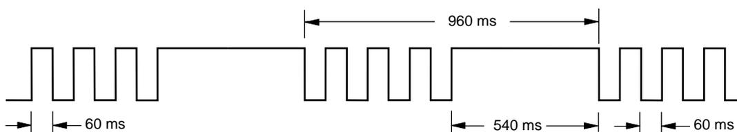
**Sensor defect, maximum values (MAXFEL - H/ MAXFEL - V)
