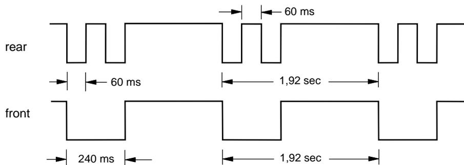
**Sensor defect, minimum values (MINFEL - H/ MINFEL - V)
