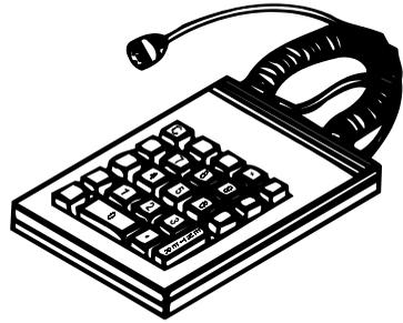
The external keypad facilitates entry of numerical values. The keypad is not absolutely essential for the program cards described in these instructions.
