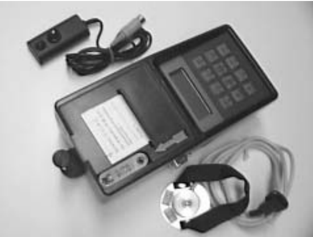
MAHA deceleration meter, type VZM 100 with pedal force meter and manual trigger
