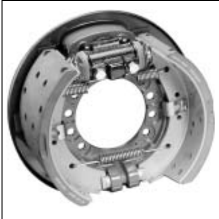
Rear axle: Simplex Expanding Wedge Drum Brake 410 × 200 ZE
