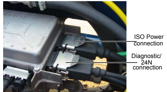
fig. 12 Socket connections and function of ISO cable
